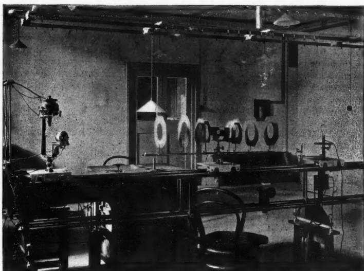
FIG. 4.—Photometer Bench for Life Tests on Glow Lamps (screens partially removed)
